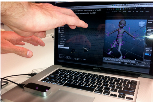
Figure 2: The midair hand gestures manipulation technique using Leap Motion and LeapStreamer
