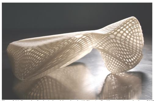
Figure 3.16: Example of a physical model produced with Sintering Rapid prototyping technology, 2007.
