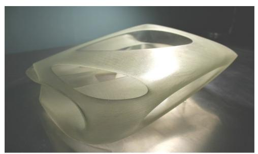
Figure 3.17: Example of a physical model produced with Rapid prototyping technology, 2007.
