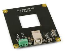
Figure 3 Phidget RFID reader
