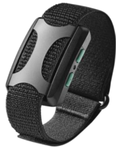
Figure 3: Apollo uses low-frequency sound waves, targeting touch receptors in the skin to send a signal of safety to sensory and emotional cortices in the brain, which rebalances the nervous system according to one’s chosen mode (Apollo Neuroscience, 2021c; 2022a; 2022b).
