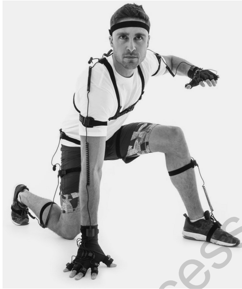
Figure 11.6 The Perception Neuron motion capture system.
