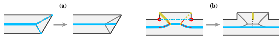
Figure 10.17: Adjustment of a blunt-tip (a) , and a T-junction with a compound split (b) . The blunt-tip disqualifies two of the branches incident to the fork (dashed blue) and the other branch is extended to reach the outline. The compound split replaces the branches associated with the split with a straight path segment. The segment is extended (dashed black) to intersect with the opposite path.
