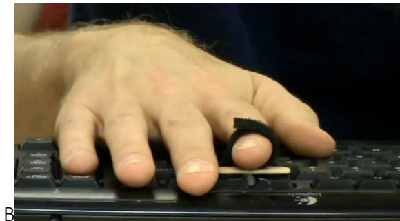
Figure 1.4. Moore and Pope's Ambiguous Movement Paradigm: A) Illustration of the pulley mechanism: A finger is fixed to a key with a Velcro strap. A pulley hidden under the keyboard can pull the key - and with it the finger - down. B) Screenshot of the video stimulus.
