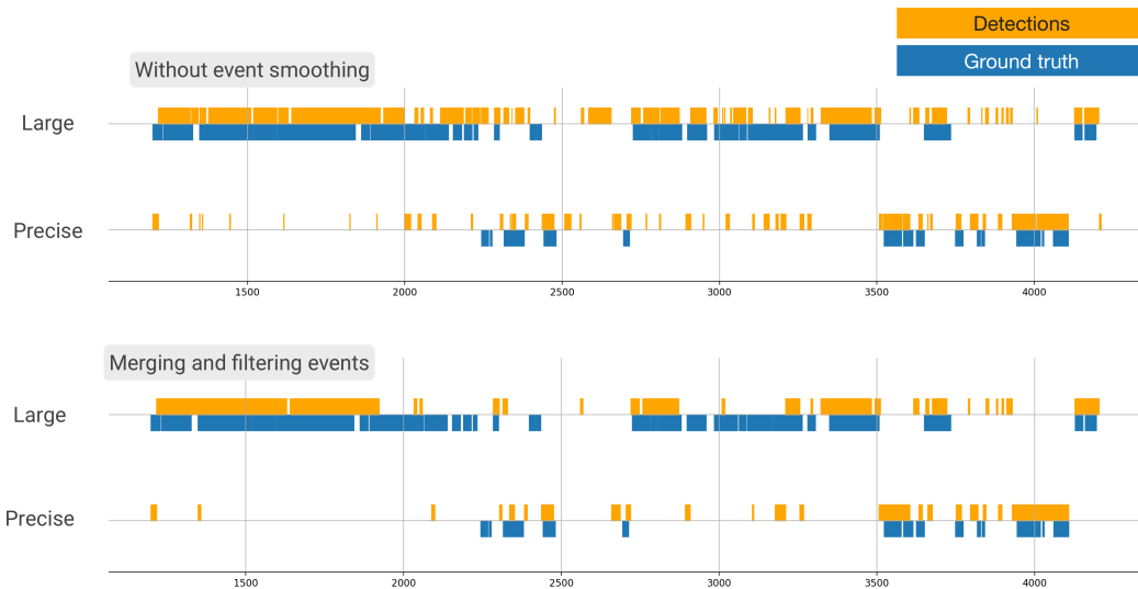
Figure 10. Ground truth events and detections for the two class problem for person two in dataset A without (top) and with (bottom) event filtering and merging. The classifier was trained using all features combined and only with data from dataset B.
