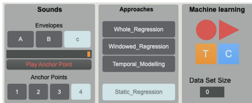
Figure 3: The machine learning training panel, with selection of sounds (with possible selection of anchor point for static regression) (Left), Selection of ML algorithm (Centre), and Record, Play, Train, and Clear Dataset buttons (Right).
