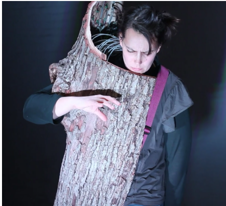
Figure 1: The MARTLET instrument, created with IML, uses gestured sensed with photoresistors to control sound.
