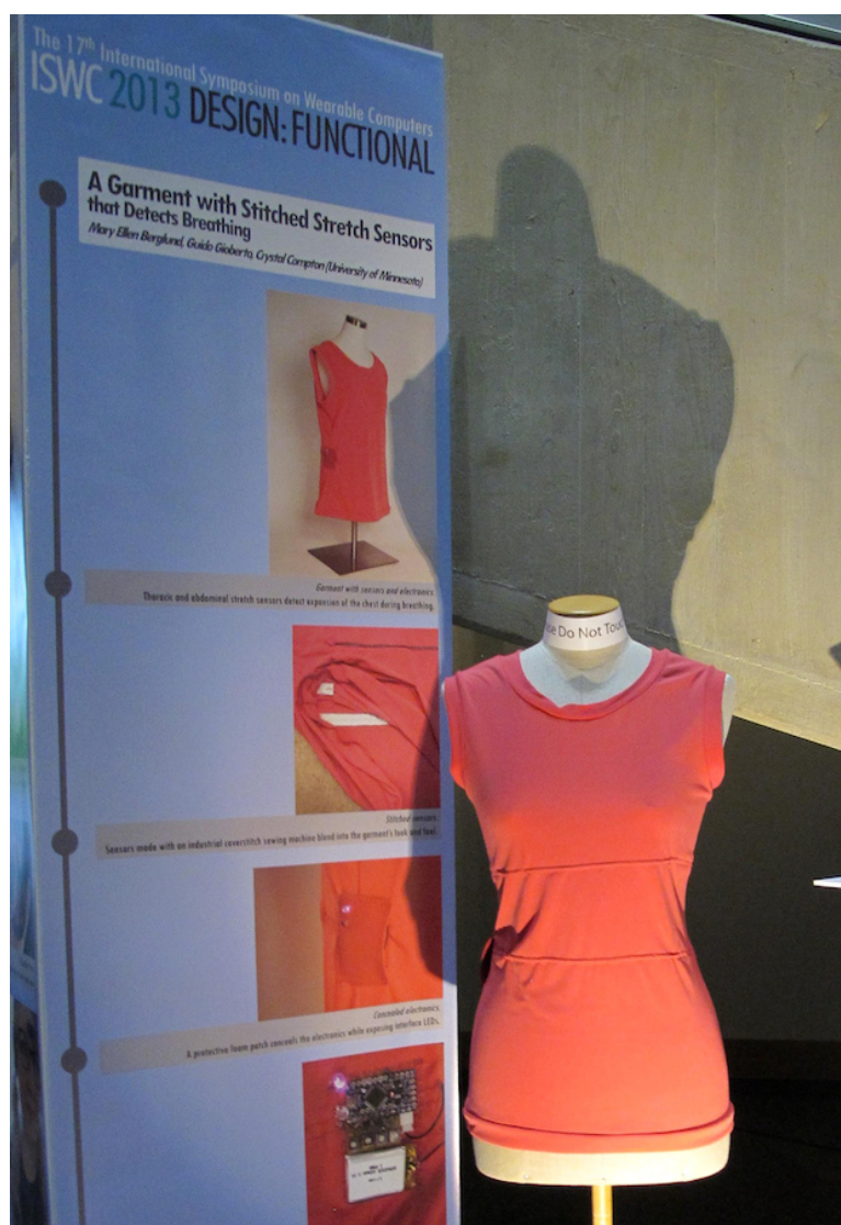
FIGURE 3.5: Garment with Stitched Stretch Sensors that Detects Breathing at the Design Exhibition, ISWC 2013, Zurich, Switzerland (2013)
