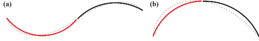
Fig. 2. Decomposing Euler spirals (stippled grey) into arcs. (a) two arcs delimiting an inflection. (b) one segment with angle > (3/4)\pi divided into two arcs.
