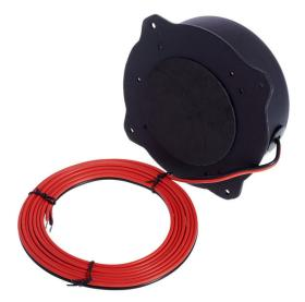
Figure 5.1: A Visaton BS130 low frequency exciter. The audio signal is transmitted to the exciter via an audio cable. Inside the exciter a driver transduces the audio signal into vibrations of a metal plate. The plate is coupled to a surface so as to resonate it and diffuse sound through the medium of the surface itself, rather than through air, as with traditional loudspeakers.
