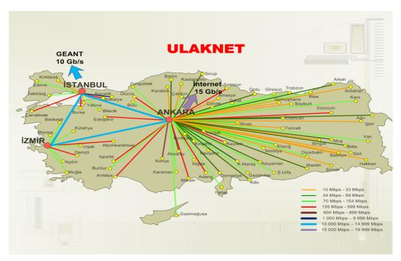
Diagram iii: network topology of ULAKNET with relative connection speeds on a national scale. *Courtesy of ULAKBIM.*
