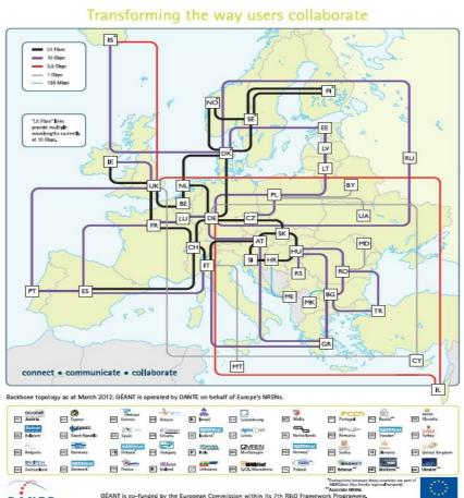
Diagram iv: Network topology of the GEANT research network. The node labelled as 'TR' represents the ULAKNET national network. *Courtesy of the GEANT project.*
