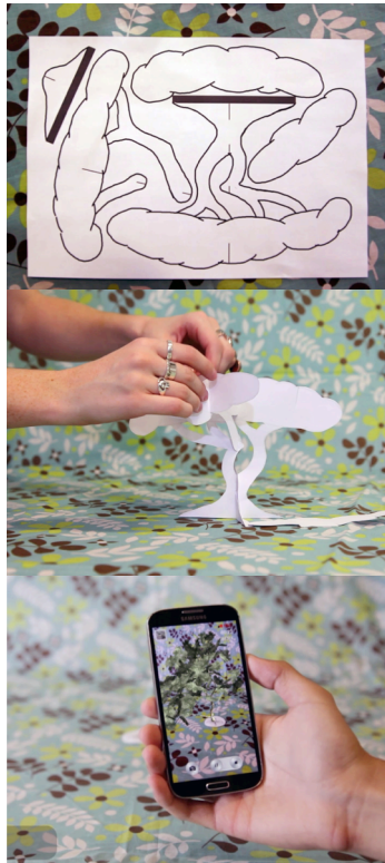
Figure 3: 3D paper tree made from 2D paper print and used as fiduciary marker to display virtual AR tree.
