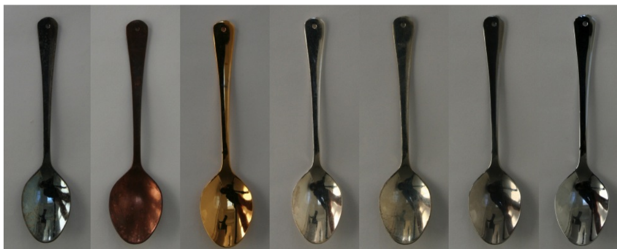
Fig. 5. The spoons material set. From left to right: zinc, copper, gold, silver, tin, stainless steel and chrome.
