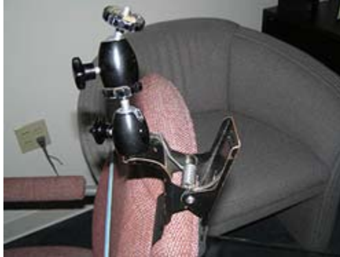
Figure A5.00.0 Modified miniature tripod clip, for attaching the camcorder to the seat in front of the cammer 753 .
