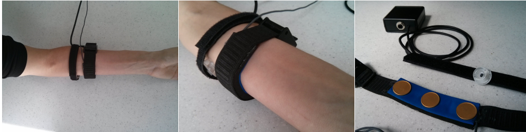
Fig. 3. Experimental setup. Left: EMG, MMG sensors placed on the forearm. Middle: EMG, MMG sensors placed on the forearm (close view). Right: Both EMG (left) MMG (right) sensors.
