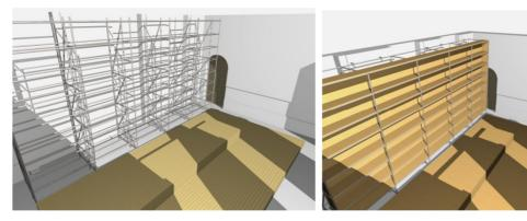
Structural Model to calculate the weight and resistance of the structure, so as to be able to insure the collection objects. Renders: Tiago Costinha
